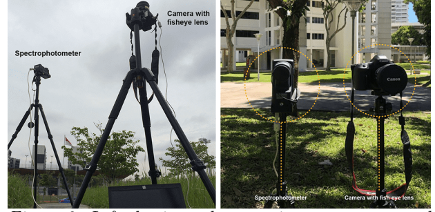
Figure 2: Left: horizontal measuring set up to record spectral measurements of sky at the open site. Right: vertical measuring setup to record spectral measurements within an urban environment.
