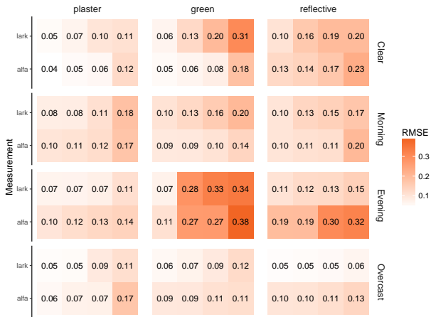
Figure 9: RMSE errors calculated as per equation (1) for LARK and ALFA multi-spectral simulations under the four sky conditions in plaster, green and reflective environments
